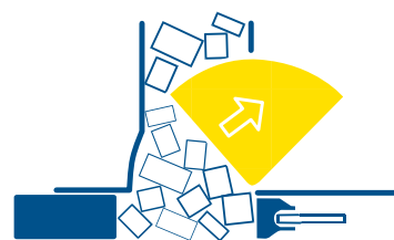
The prepress opens and the material stacked on top of the pre-press falls down into and fills the press chamber.
