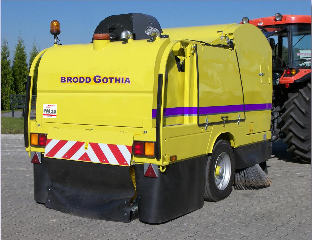
Gothia elevator sweeper can be equipped as option with an effective suction fan for collection of the fine dust, created during the sweeping.
