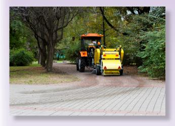
**Side displacement of the draw bar Twiggy** is as standard equipped with a hydraulic left/right displacement of the draw bar. It is remote controlled with joystick. The flexibility in curves and around e.g. poles gets even better and You can simply sweep "every corner" clean.
