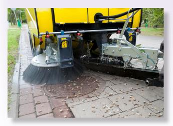
**Sprinkler system** The water sprinkler system helps to prevent the dust around the sweeper.
