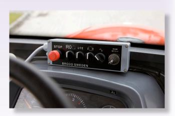
**Remote control** All sweeping operations are operated from the driver's cab. Sweeping on/off, water pump on/off, dirt hopper up/down etc.
